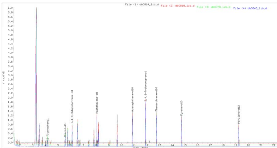
Figure 2: Overlay of chromatograms from multiple samples from 10 home survey. Peaks with names are surrogates and internal standards.
