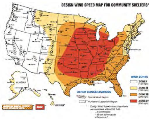
The “Design Wind Speed Map for Community Shelters” is one way of graphically analyzing wind risks. As can be seen, all of the counties in the region are in a “Zone II” with respect to design wind speeds, which means that shelters constructed for protective purposes should be designed to withstand up to 160 mph winds.
