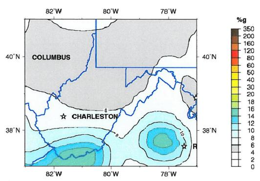
Peak Acceleration (%g) with 2% Probability of Exceedance in 50 Years site: NEHRP B-C boundary National Seismic Hazard Mapping Project (2008)
